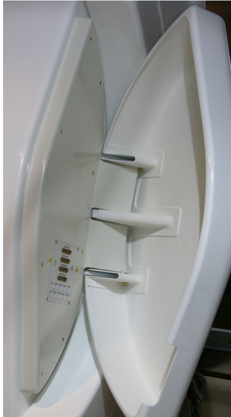
Fig. 1.12. The electrode interface panel is under the gantry side cover.
