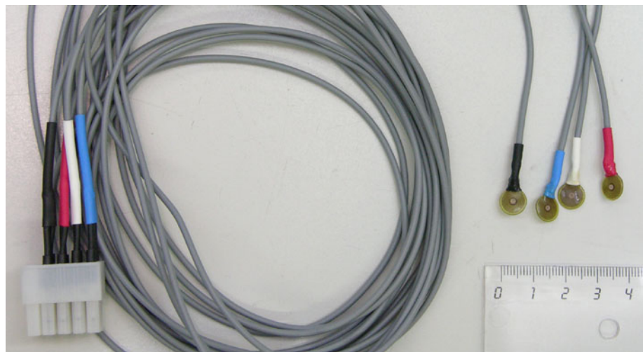
Fig. 1.16. Head position indicator coils.
