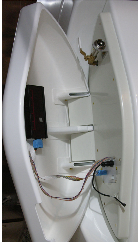
Fig. 1.19. The auxiliary electronics panel is under the gantry side cover. The liquid Helium level meter local display is mounted on the cover. Microphone for the optional intercom is seen in lower right corner.
