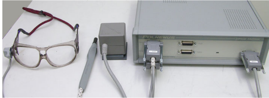
Fig. 1.17. 3-D digitizer unit. The transmitter coil (closest to the unit), digitizing pen, and goggles with separate reference receiver (leftmost) are also shown.
