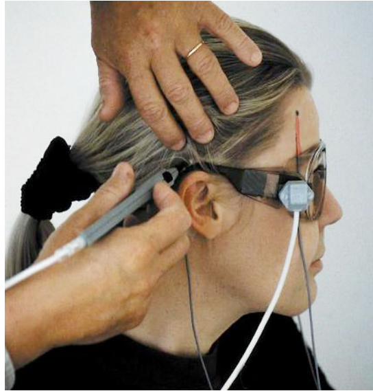
Fig. 3.4. The head digitization goggles with additional receiver.
