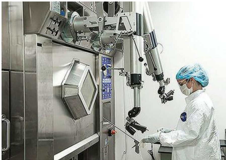
Figure 11.4 A cyclotron facility used to produce positron emitting radioligands (PERs) used in PET scanning. Radioactive materials are kept inside the heavily shielded container on the left, with the necessary apparatus for the technician to manipulate and view the process safely outside the shielding on the mechanical arms in the centre of the picture. Image used with permission of Lawson Health Research Institute, London, Ontario, Canada
